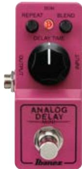
With its ultra-compact size, the **Analog Delay Mini** packs true analog delay tone into a pedal that can squeeze onto the most cramped of boards. You'll be able to dial in everything from short slapbacks to echoes, with the 20ms–600ms delay time range. The signal path is 100% analog, and true bypass switching completely takes the effect out of your guitar's signal path when disengaged.
