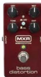
MXR's **M85 Bass Distortion** is a 2-voice pedal that distorts your highs and leaves your lows tight and punchy. Not only can you dial in the tone of the distortion effect, but you also get your choice of aggressive silicon diode clipping with a touch of compression or the more open sound of LED distortion.
