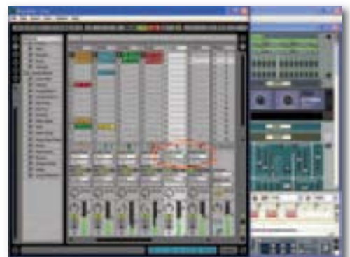
This shows Propellerhead Software's Reason ReWired into Ableton Live. Note how Live mixer channels 8 and 9 have their inputs set to monitor Reason (circled in red for clarity).
