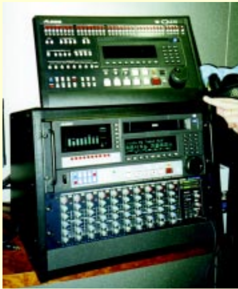
Coming soon to a rack near you: the Alesis M20 20-bit digital multitrack. On top, the very cool new CADI remote controller.
