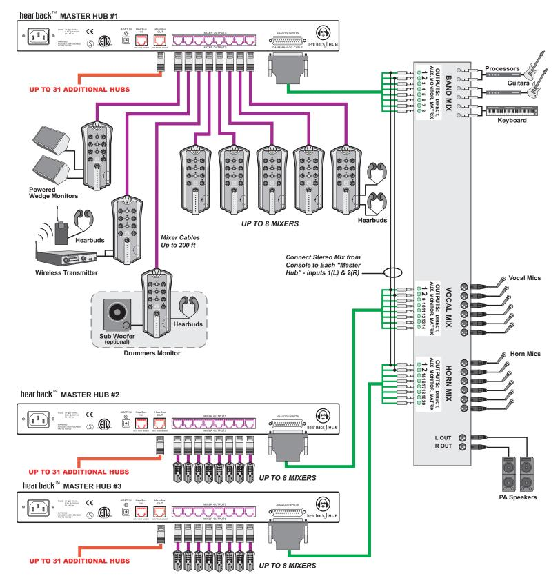
NOTE: Each hub gets the stereo mix and sectionals. Each master hub can have 31 hubs daisy-chained from it.
