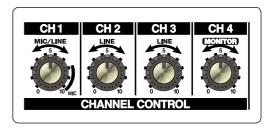
Adjust the volume balance for channels 1 through 4 at this time.
