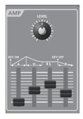
The AMP section contains parameters that control the volume. Raising a value will increase the volume.
