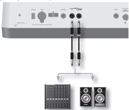
\* In order to take full advantage of the GAIA SH-01's capabilities, we recommend that you use it in stereo. To use it in mono, connect to the OUTPUT L/MONO jack.
