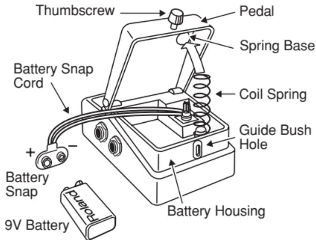
**1.** Loosen the thumbscrew at the front of the pedal, then lift the pedal upwards to open the unit.
