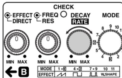
1. When you have made the necessary connections (p. 8), set the knobs as shown in the illustration.
