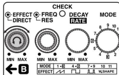
7. Adjust the volume of the effect and direct sounds using the EFFECT Level and DIRECT Level knobs.
