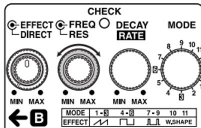
6. Adjust the feedback amount of the filter using the RES knob.
