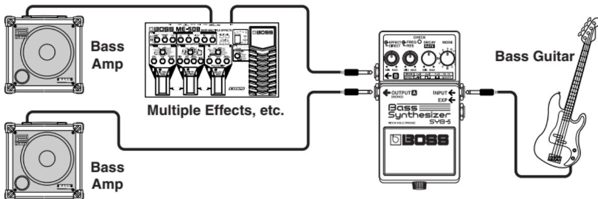
*\*To ensure stable conditions, connect the SYB-5 directly to your bass's output. Connect any additional effects to the SYB-5's OUTPUT A (MONO) or OUTPUT B jacks.*
