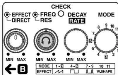
5. Adjust the frequency of the filter using the FREQ knob.
